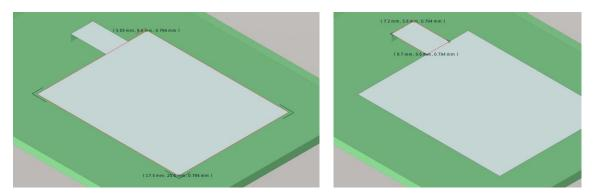
This antenna is placed on a substrate with  $\epsilon_r = 2.2$  and the height of h = 0.794 mm (RTDuroid). The substrate is a  $40 \times 40 mm$  square. Draw/simulate the antenna in the simple (plane) model with PEC <u>and</u> in the technologic accurate version with 0.1mm copper metallization on the same type of substrate and passivation with 0.01mm Si<sub>3</sub>N<sub>4</sub> (materials from the Standard Material Library).
