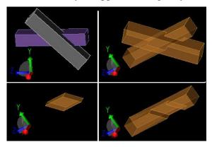
It is essential that no overlapping objects remain in the drawn structure (for example, an dielectric object and a metallic object cannot coexist in the same point in space). As such, Boolean operations between objects are either optional (as a method of drawing complex objects that cannot be described with elementary 3D blocks) or mandatory to remove illegal overlaps between objects.
