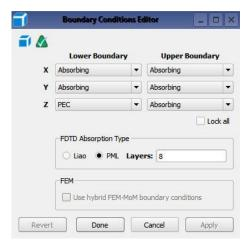
The most common values are Absorbing (equivalent to free space, all energy exits, nothing returns), PEC (perfect electrical conductor - equivalent to the ideal metallic wall), PMC (perfect magnetic conductor - mathematical idealization, usable for odd symmetry of electromagnetic fields), Periodic (means the infinite repetition of the structure, usable for periodic structures - instead of simulating thousands of identical cells we can simulate only one).
